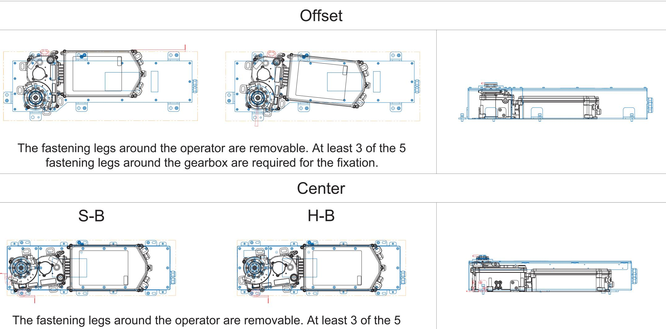
fastening legs around the gearbox are required for the fixation.
